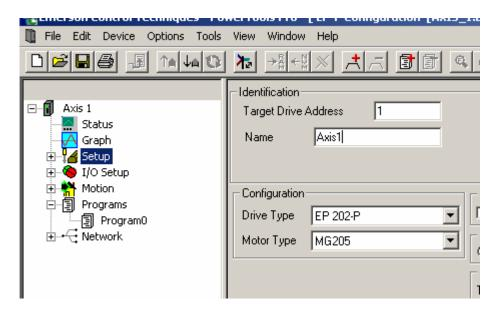
2) Within in PowerTools Pro create the list of modbus variables that are to be read/write from the CTVUE HMI.Click the
